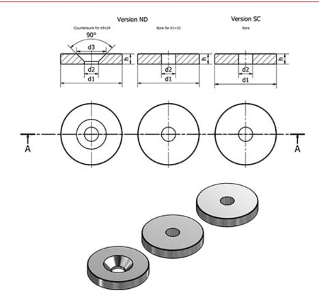
$\begin{array}{lll} \text{d1} & = 15 \\ \text{d2} & = 8 \\ \text{d3} & = - \\ \text{h} & = 3.5 \\ \text{Nominal adhesive forces in N} = 23 \end{array}$
